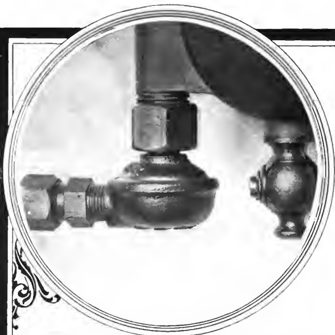
Fig. 6—Point of entrance of the gasoline to the carbureter, showing the filtering device and pipe connections
